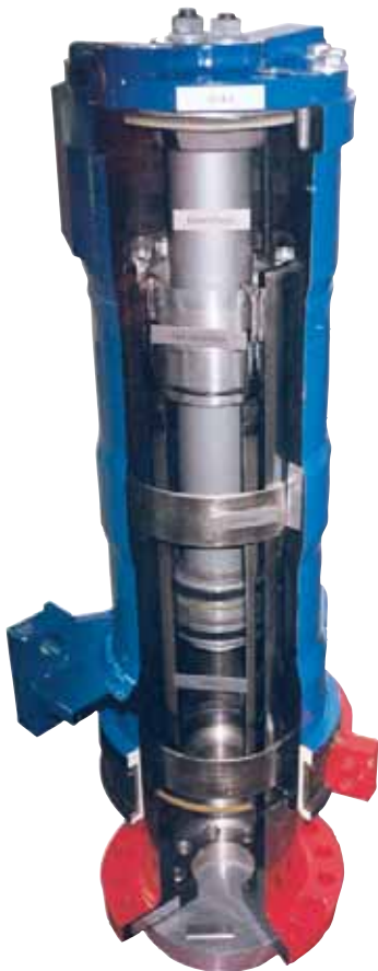
A cross-section showing the inside of a Megastrut.
