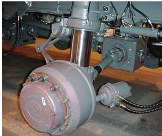
Detail of the Megastrut, which removes the need for conventional axles.
