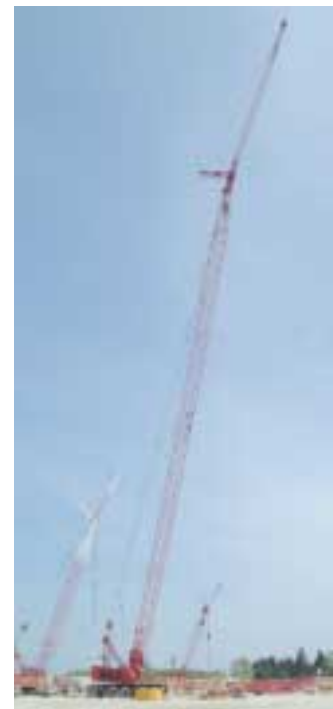
A maximum of 58 m (190 ft) of main boom and 18 m (60 ft) of jib can be fitted to the Model 222 Wagon.
