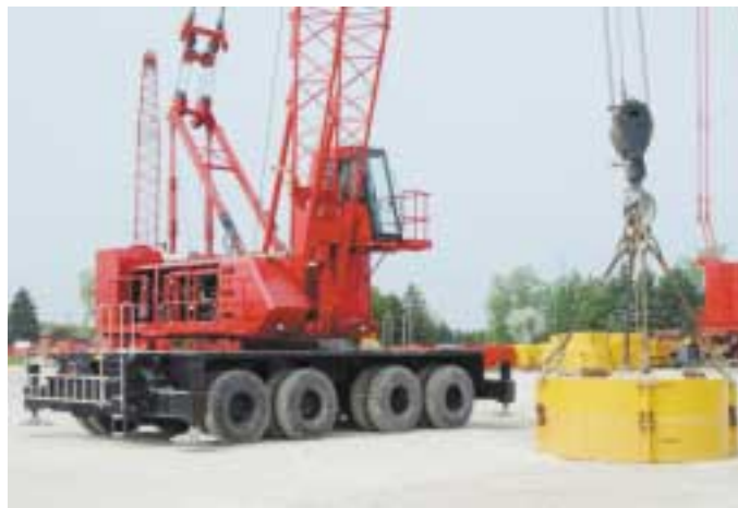
For dockside work the unit can be fitted with an elevated cab.
