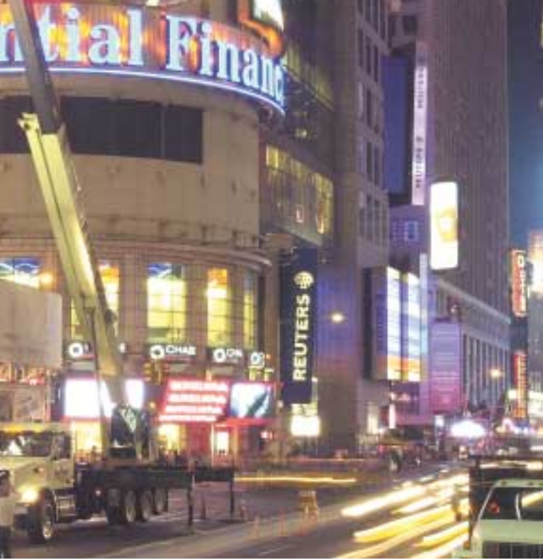
A National 1800 series boom truck lifts a 9.1 m (30 ft) piece of a Jack-and-the-Beanstalk sculpture onto the corner of a building in Times Square, New York City. The 36 t (40 USt) capacity crane is capable of reaching a 53 m (175 ft) tip height with its swingaway jib fitted. The crane is owned by Five Boro Boom Service of Maspeth, Queens, NY.
