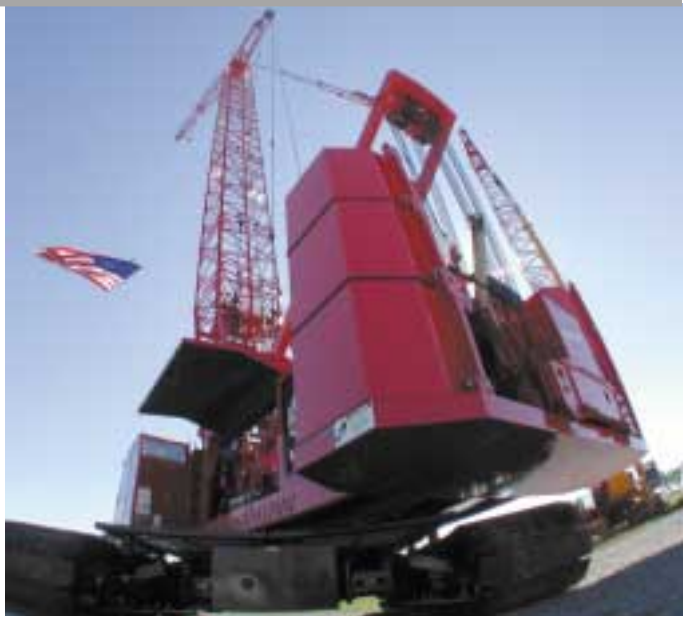
The Manitowoc Model 555 crawler crane was shown with its luffing jib for the first time.
