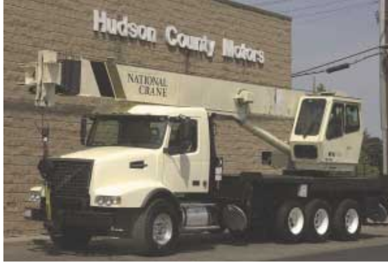
A National 1400 series boom truck with a swing cab on a Volvo chassis outside Hudson County Motors in Secaucus, NJ. The 30 t (33 USt) capacity unit has a maximum tip height of 50 m (164 ft).
